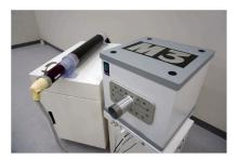
The M3<sup>™</sup> compact MRI System may be paired with Brightonix Imaging's preclinical positron emission tomography (PET) system, which is based on advanced silicon photomultiplier (SiPM) technology, to provide excellent sequential imaging performance for PET/MRI preclinical studies.
