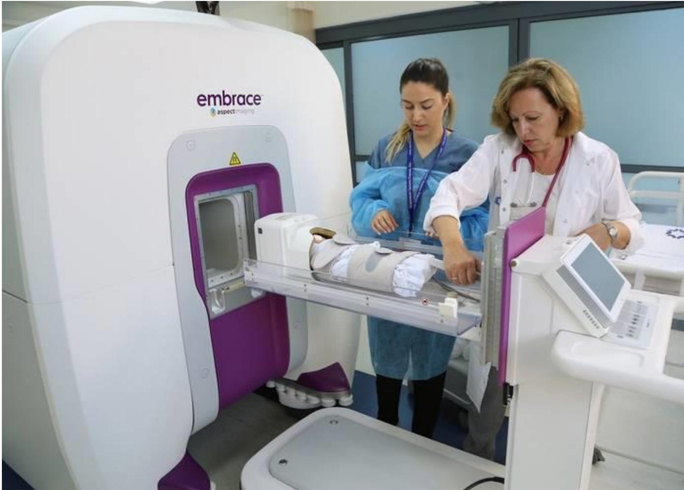
The new Embrace MRI system for infants at Brigham and Women’s Hospital in Boston makes it easier to monitor brain development. It has a temperature-controlled incubator to minimize the baby’s movement and makes a fraction of the noise of ordinary MRI machines. Photo: Eastside Studio
